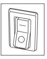
The valet lockout switch is located inside the glove box.
